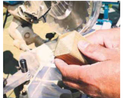
STEP 6. Once all four cuts are made, you should end up with a pointed top
